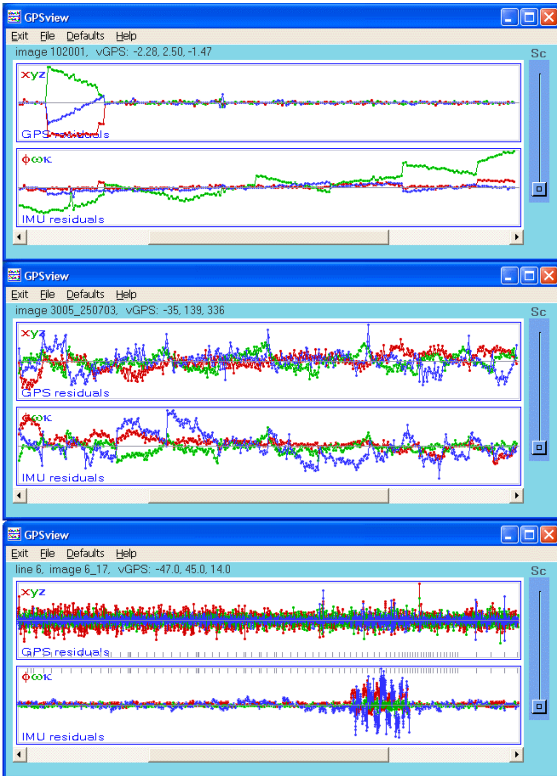
Figure 9. GPS/IMU residuals of different projects. Systematic effects and relations between GPS and IMU data can be easily identified.
